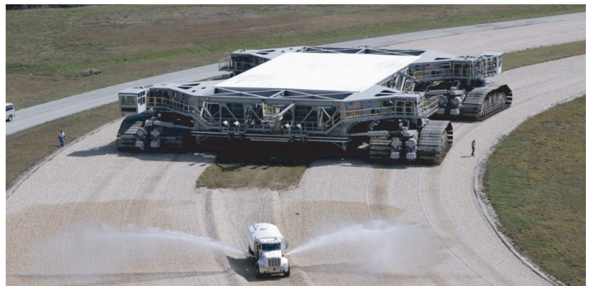
Crawler-transporter responsible for moving rockets and spacecraft to the launch pad at NASA's Kennedy Space Center in Florida for over 60 years.
