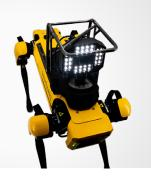
Enterprise asset management programs now have a high volume, highly repeatable route-based vibration analysis solution with dynamic mobility and teleoperation capabilities. Measuring deflection, displacement, movement, and vibration not visible to the human eye autonomously, Iris Explorer minimizes risk, helps maintain compliance and increases asset ROI for improved asset reliability and performance.
